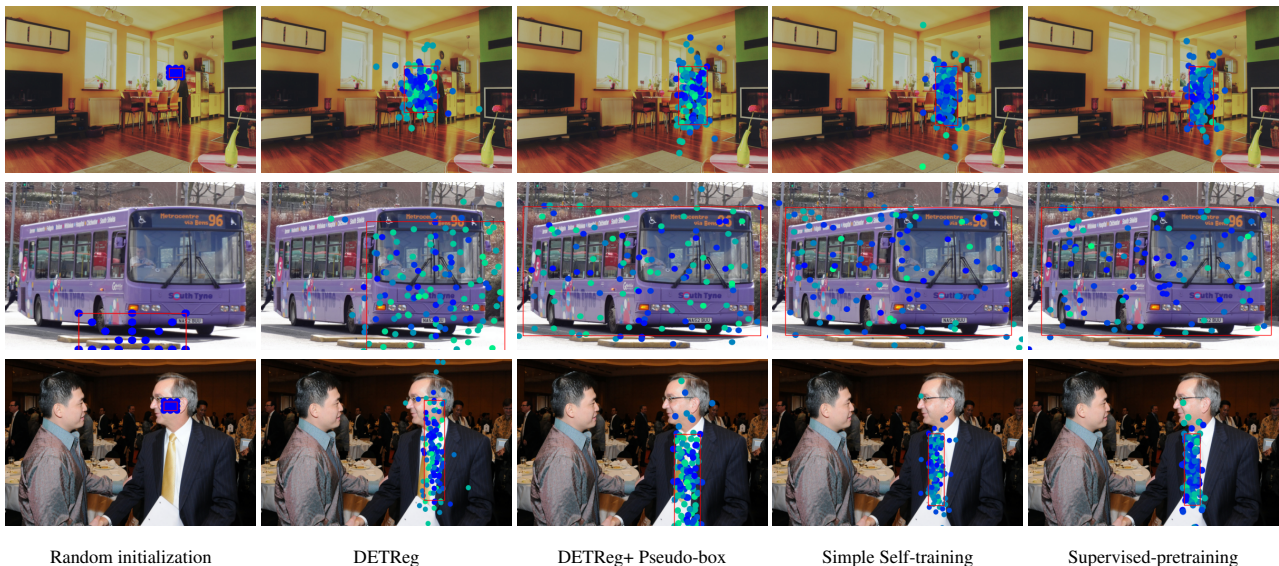
Fig. 7: Visualizations of deformable cross-attention based on the last Transformer decoder layer on COCO val images.
